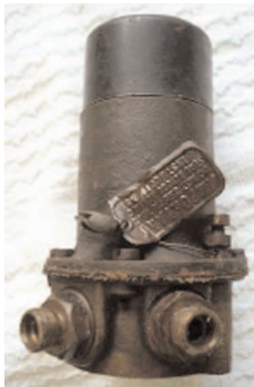
Fig 1 – Photo of a very early brass based pump with its seal and label intact. The label reads: “IMPORTANT DO NOT BREAK THIS SEAL BEFORE READING THE INSTRUCTIONS.”
